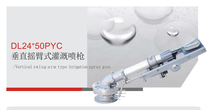
DL24°50PYC vertical rocker arm irrigation spray gun adopts the form of double rocker arm. The vertical rocker arm is equipped with a two-way guide plate, which rotates forward and backward through the action of water flow to different directions of the two-way guide plate, so as to realize a continuous spraying mode that can be sprayed normally both in the positive direction and in the negative direction.
